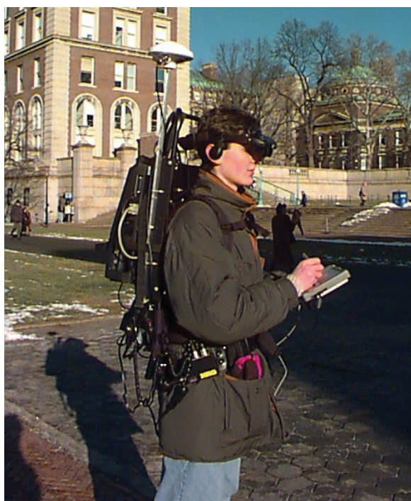
FIGURE 5.3 Prototype 3D mobile augmented reality. SOURCE: S. Feiner, B. MacIntyre, T. Hollerer, and A. Webster, A touring machine: Prototyping 3D mobile augmented reality systems for exploring the urban environment, pp. 74-81 in First IEEE International Symposium on Wearable Computers , 1997, doi:10.1109/ISWC.1997.629922. Courtesy of Steven K. Feiner.
